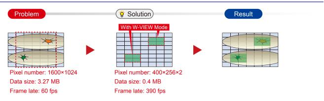
Fast experiments can generate a lot of data. What if you need to go fast but not necessarily keep every single pixel of the image? The ability to specify two regions of interest on the ORCA-Flash4.0 LT means both a big increase in speed and smaller files sizes. High-speed, extended time course data are recorded with more simplicity than ever before.
