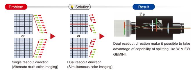
With the independent readout direction, synchronous illumination of two different wavelength is possible to image two-wavelength excitation/ two-wavelength emission simultaneously by the W-VIEW GEMINI.
