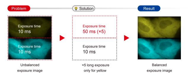
It's pretty rare that the signals from dual wavelength fluorescence samples warrant the same exposure times. When your cyan channel is screaming but your yellow is ho-hum horrible, the LT's new W-VIEW Mode takes away the need for complicated tweaks in optics or filtration and seamlessly ensures more balanced exposures for reliably quantitative dual wavelength imaging.
